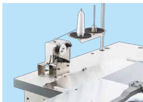
Constant-quantity bobbin thread feeding mechanism
