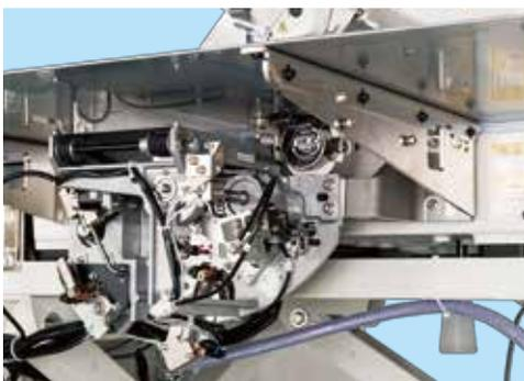
Automatic bobbin-thread winding and feeding unit
